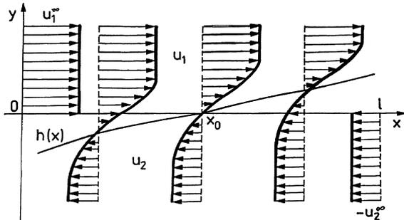
Fig. 1. Counter-current flow.
